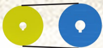
The belt on the first driven pulley. Position 1: slower driving, but stronger power.
