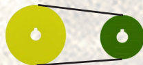
The belt on the second driven pulley. Position 2: the car goes faster
